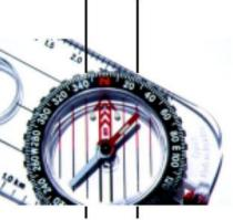
Turn the compass housing until the red arrow on the base plate points to the top of the map. Line up the orienting lines on the base to the grid lines on your map. They should rest on top of or be parellel to the grid lines on the map. Again be precise as possible.
