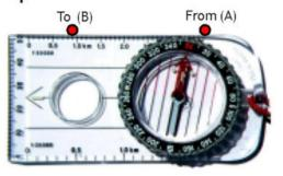
Start by placing your compass on the map. Place the edge of the compass along the line you wish to travel from A - B. Do this as precisely as possible and if possible each location should be a recognisable feature - fork of a stream to edge of forest. The direction of travel arrow should point in the direction you wish to travel (A - B)
