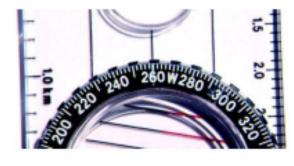
Lift the compass from the map and read the bearing indicated on the housing by the direction of travel line. Say this reading to yourself "260 degrees plus 10 degrees equals 270 degrees". 10 degrees are added for magnetic variation in Ireland. (This figure can vary so check map to find correct variation for your area.) It is best to confirm in your mind what the final bearing is before you move the compass housing.
